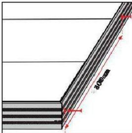
The spacing between the screws should not exceed 300 mm. Allow a minimum 6 mm gap between the fascia and any vertical walls or the ground for drainage.
